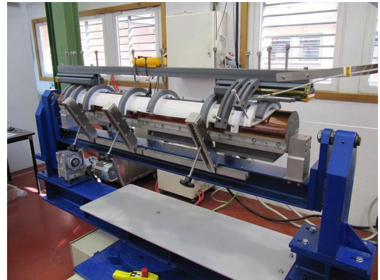
Winding of the first coil at CIEMAT (F. Toral)
