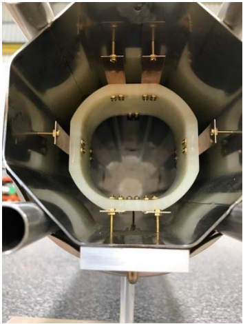
Displacement measurement tooling (Courtesy Oscar Sacristan De Frutos)
