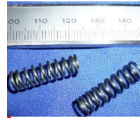
20 titanium G5 springs (total prestress: ~360 N)
