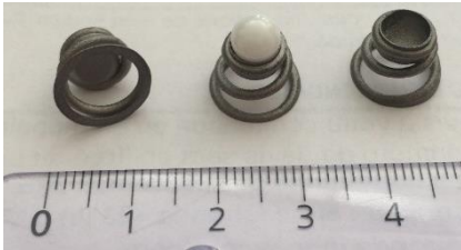
3D printed titanium spring with ZrO2 ball
