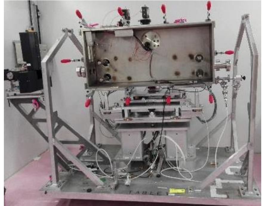
The opened vacuum vessel with jaws removed
