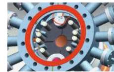
Example of diagnostic box at RHIC e-lenses
