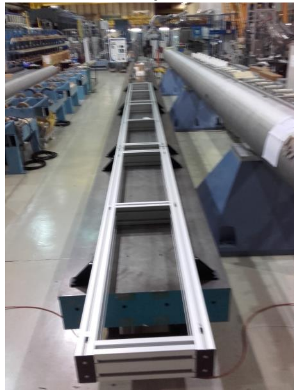
MQXFB magnet and cold mass Assembly bench
