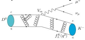
$$\begin{split} \frac{d\Gamma}{dq^2} &= \frac{G_F^2 |V_{cs}|^2}{8\pi^3 m_D} |\vec{p}_K| |f_+^K(q^2)|^2 (\frac{W_0 - E_K}{F_0})^2 \\ &\times \left[ \frac{1}{3} m_D |\vec{p}_K|^2 + \frac{m_\ell^2}{8m_D} (m_D^2 + m_K^2 + 2m_D E_K) \right. \\ &+ \frac{1}{3} m_\ell^2 \frac{|\vec{p}_K|^2}{F_0} + \frac{1}{4} m_\ell^2 \frac{m_D^2 - m_K^2}{m_D} \mathrm{Re}(\frac{f_-^K(q^2)}{f_+^K(q^2)}) \\ &+ \frac{1}{4} m_\ell^2 F_0 |\frac{f_-^K(q^2)}{f_+^K(q^2)}|^2 ] \end{split}$$
