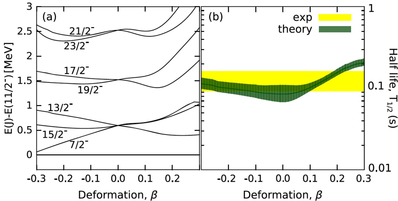
Level ordering and lifetime measurement constrains deformation of  $^{151}\text{Lu}$  to be mildly oblate  $\beta = -0.11(2)$
