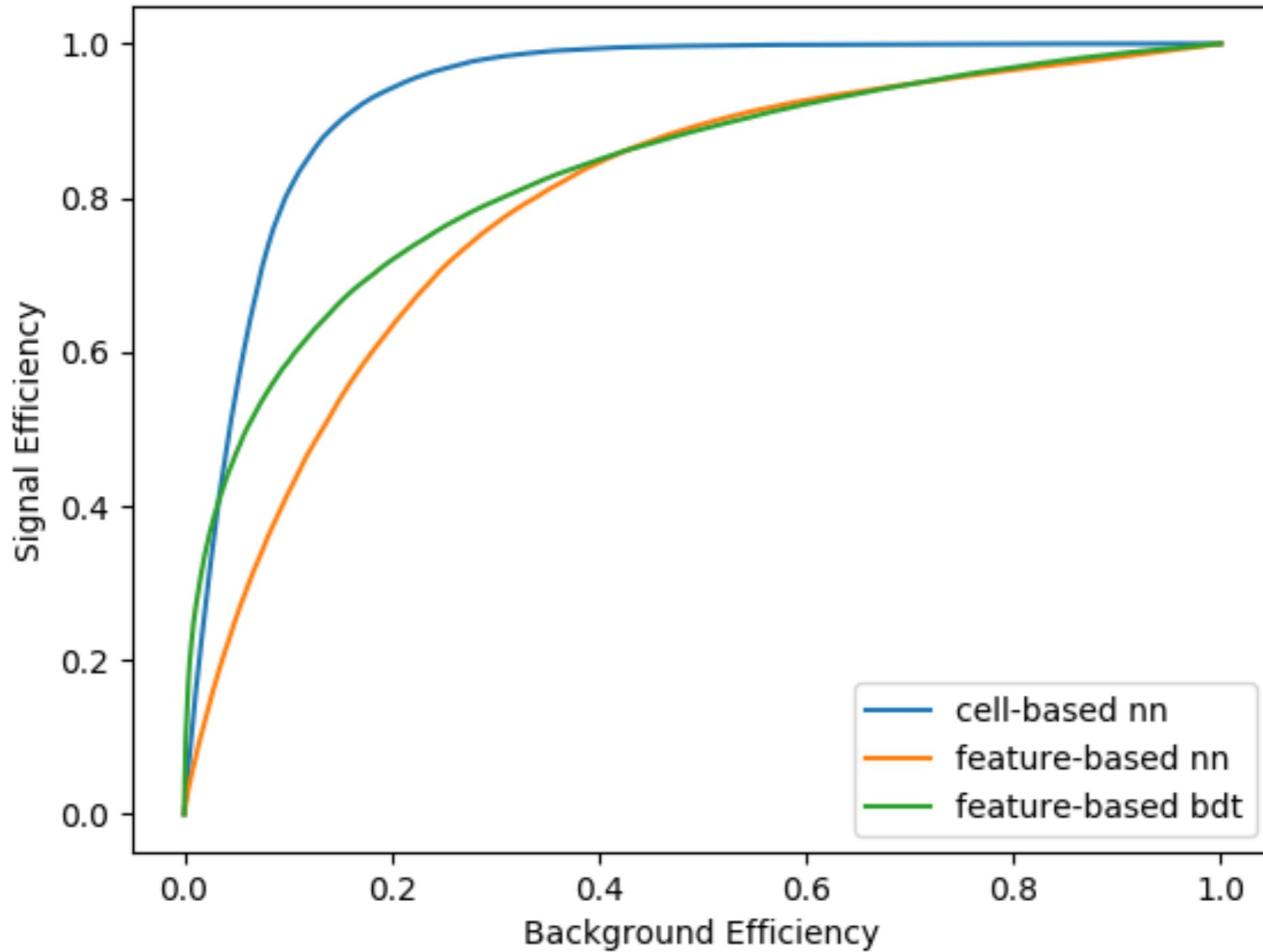
**0.2 increase in signal efficiency, 15 increase in back efficiency**
