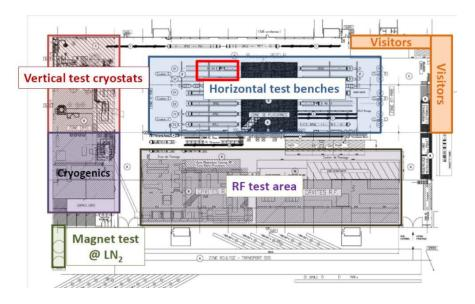
Superconducting magnet coil prototypes can be tested in the vertical cryostats. Horizontal test benches are designed to qualify complete magnets with cryostats. The RF area serves for testing superconducting RF cavities. To shield operators from the X-rays generated from new cavities, they are housed in concrete bunkers.
