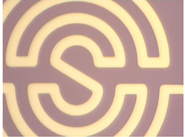
Metallic line for 200 \Omega coiled RTD with evaporated metal deposition at 100x zoom.
