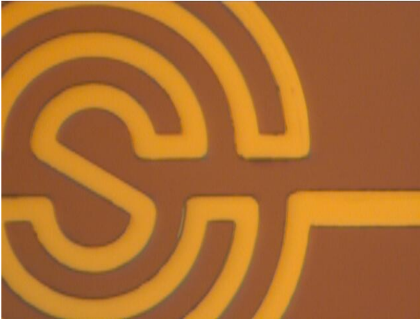
Metallic line for 200 \Omega coiled RTD with sputtered metal deposition at 100x zoom.
