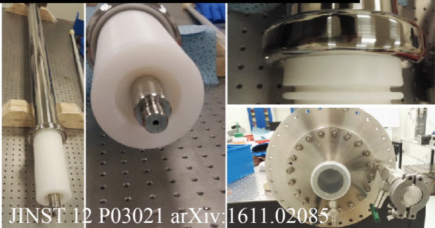
Sept : Test & insertion of 300 kV HV feedthrough
