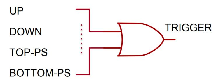
➤ Final trigger provides gate for ADC, common stop for TDC, and gate for RPC Local Station
