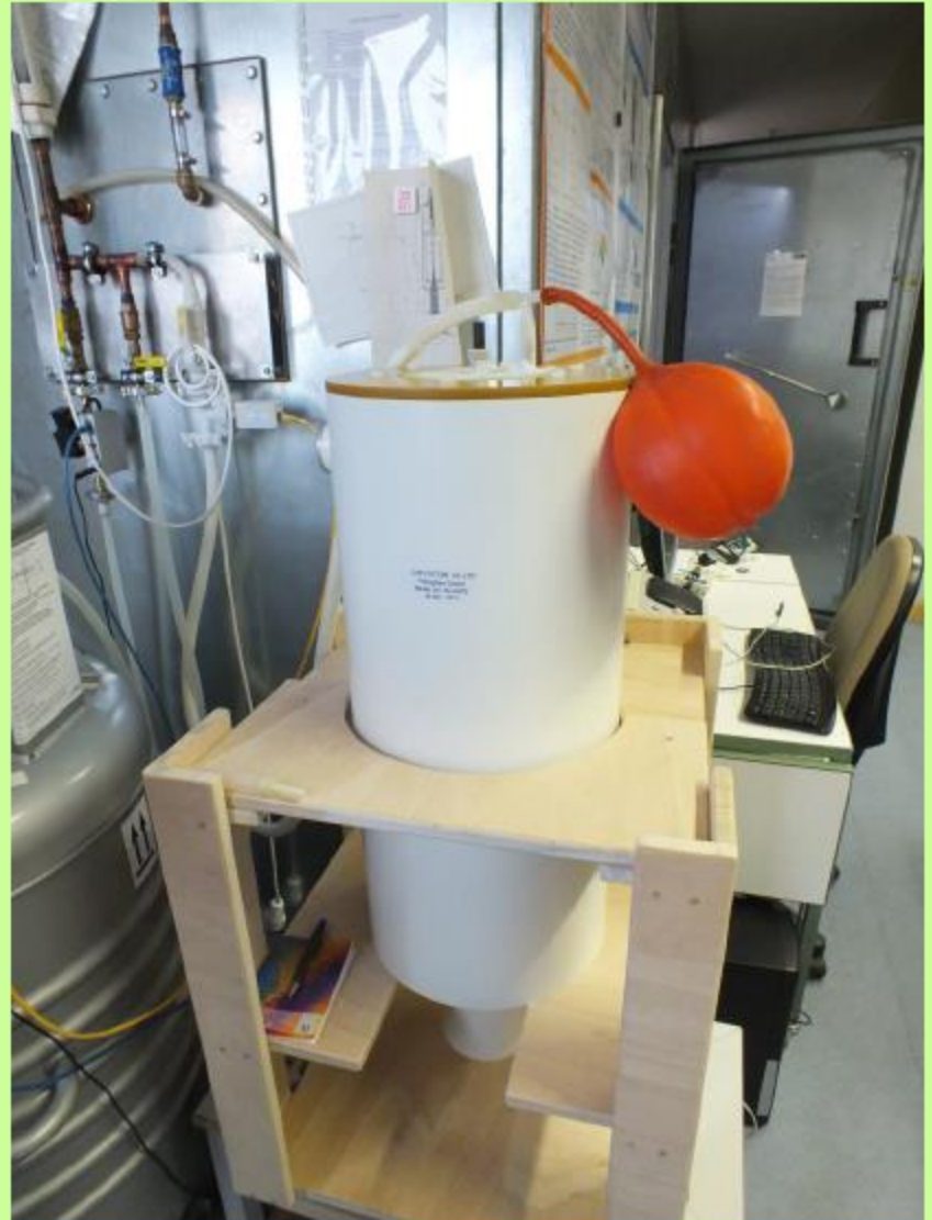
Non-magnetic ^4\text{He} Dewar housing three low- T_c SQUID gradiometers
