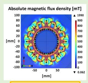
Neutron spin flipping requires magnetic field compensation
