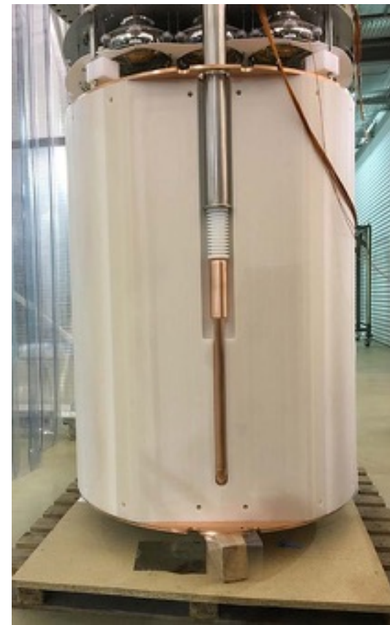
Installed HV FT
