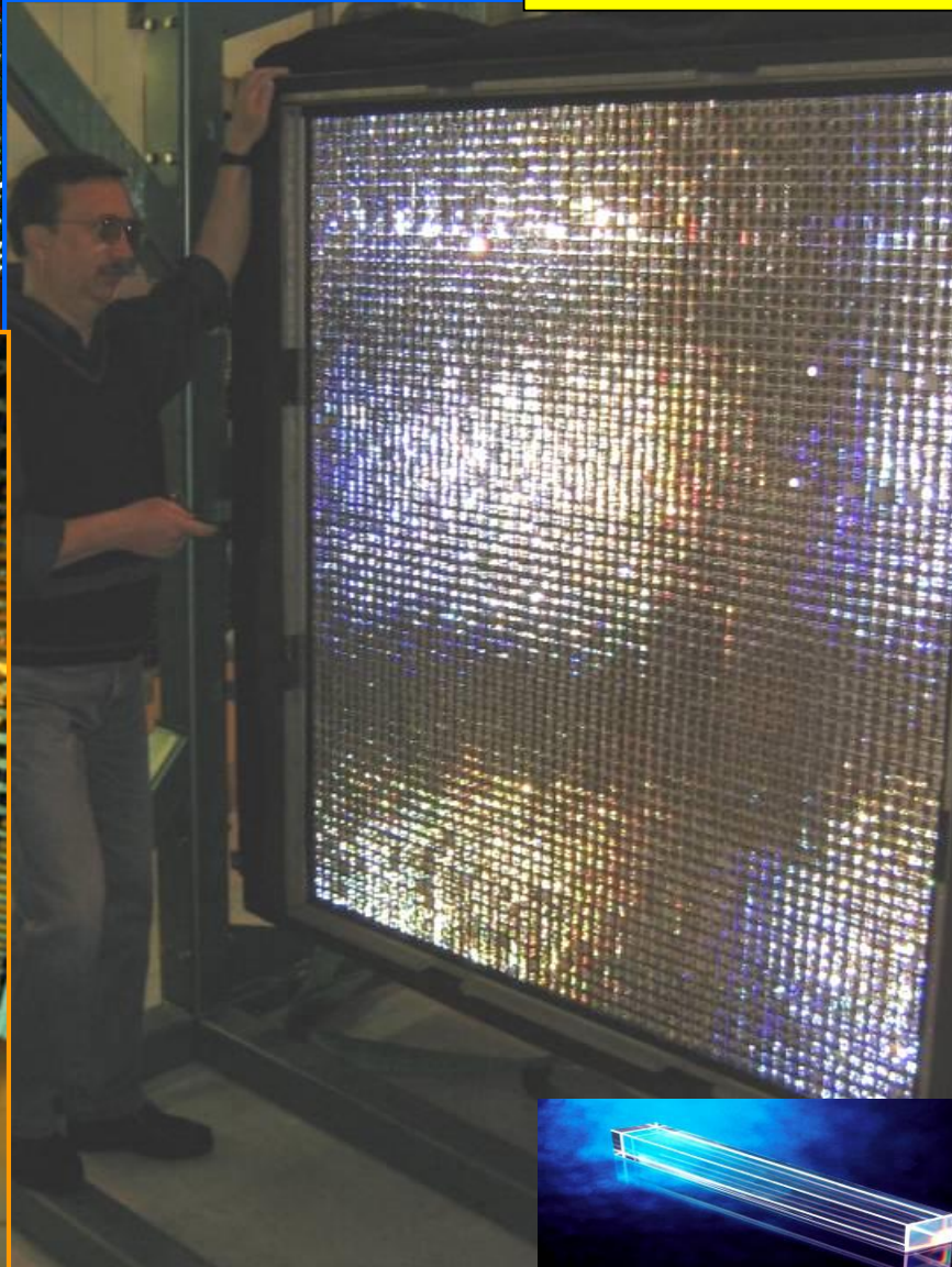
PHOS module ~ 20,000 PbWO 4 crystals
