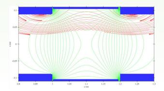
Depending on the energy and emission angle fraction of electrons are either repelled or transported over the PU
