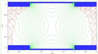
Electrons with energy below the bias voltage are repelled
