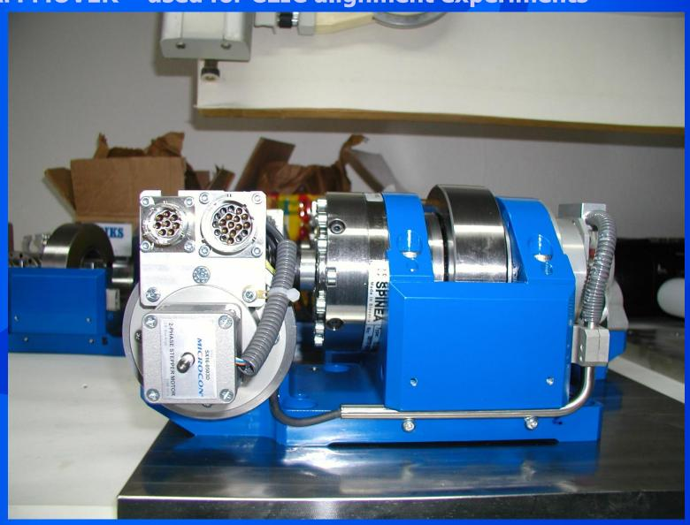
CAM MOVER – used for CLIC alignment experiments, + / - 1um positioning precision was reached
