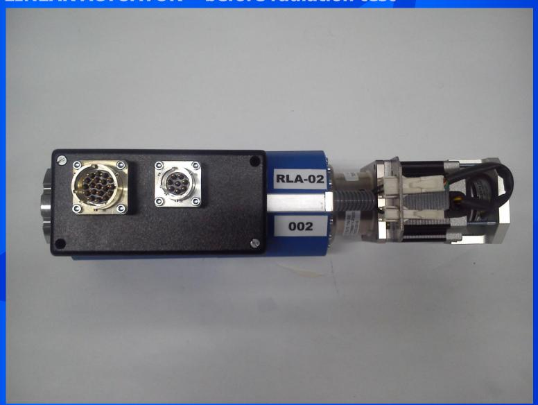
LINEAR ACTUATOR – after radiation test / 10 years cumulated
