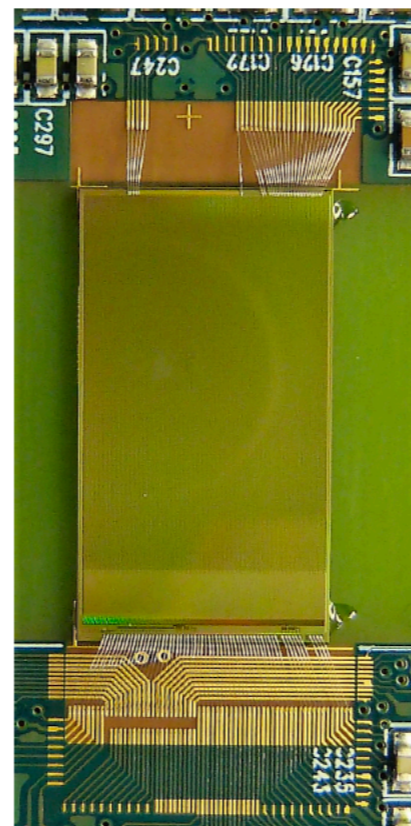
Large MuPix sensor: 2 \times 1 \text{ cm}^2
