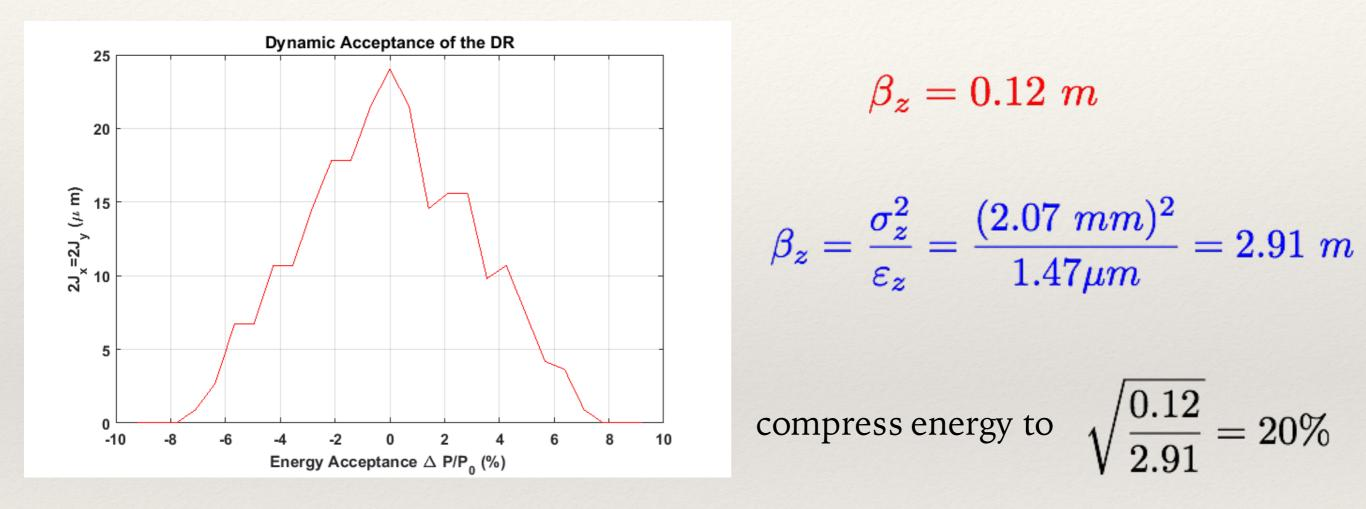
in other words, the total energy spread of e+ data should be compressed from  $\pm 12\%$  to  $\pm 2.2\%$ .
