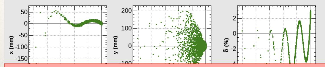
Eventhough the transverse and longitudinal matching are made, the filamentation is still apparent!
