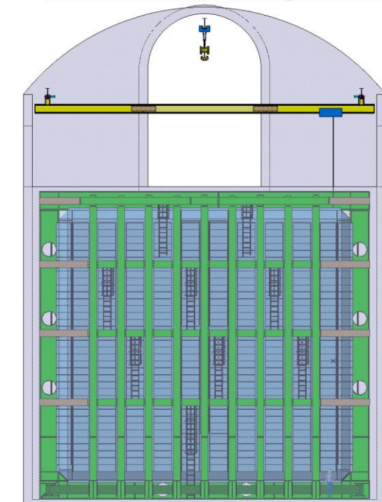
An overhead crane (under study) seems essential for realistic handling and to reduce assembly time
