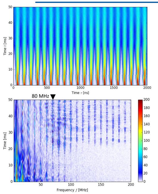
Modulation starting around t = 25 ms, if at least two 80 MHz cavity gaps are open (C80-08 and C80-88 in this case)
