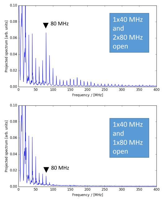
The projected spectrum is the maximum spectral components at each frequency during the acquisition (50 ms)
