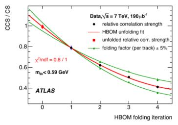
Data from the 2010 ATLAS low-mu sample; the measured value of CCS/CS corrected for detector effects by doing 3 iterations of folding through detector simulation, and extrapolating back the fitted functional form once more wrt the measured data point
