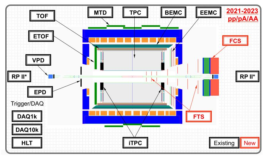
\* FTS: Forward Tracking System; FCS: Forward Calorimeter System
