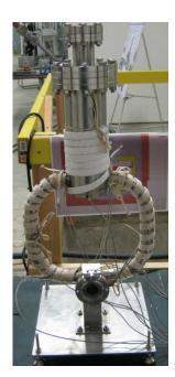
✓ Liquid Metal Target Lead-bismuth eutectic compound
