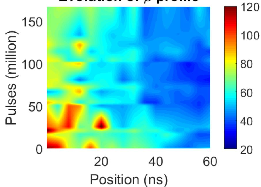
$\beta$  value corrected for varying E-field along structure.
