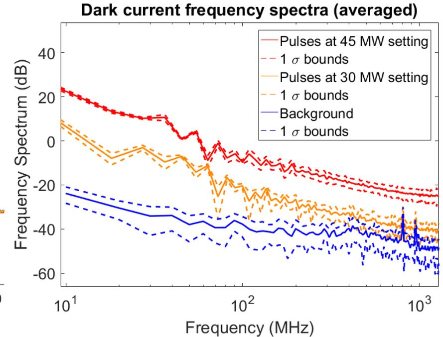
Signal is inverted and high-pass filtered by amplifier. (Passband 20 MHz – 4 GHz)
