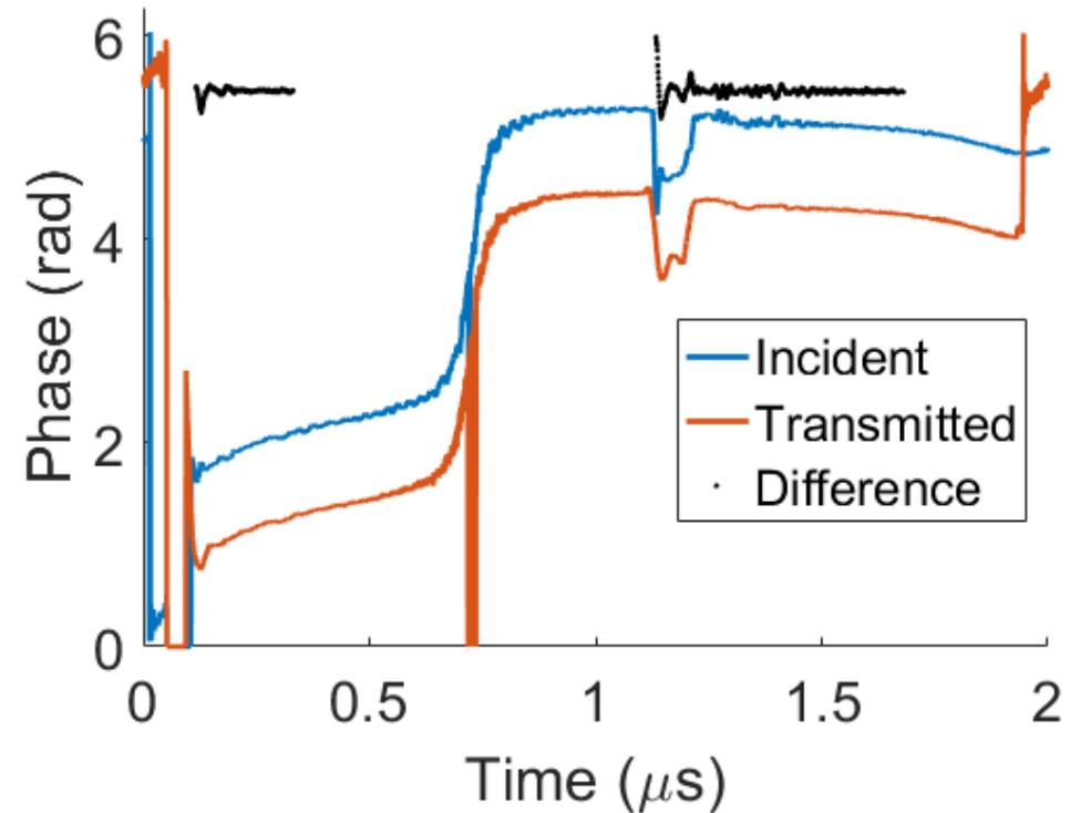
Signal edges aligned in time to compensate for time delay between incident and transmitted – important for short pulses.
