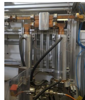
Pulse compressor: provided by CERN
