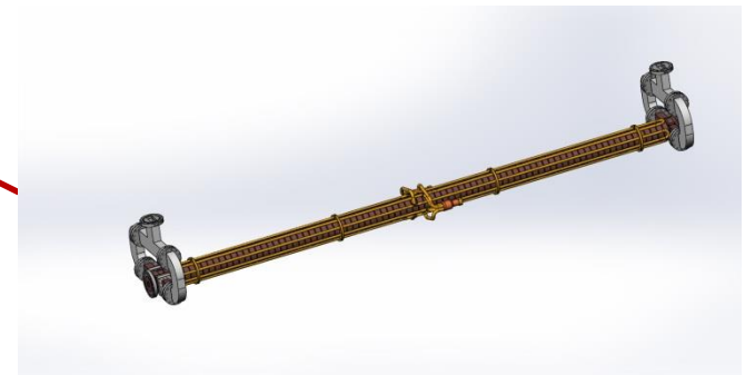
Two 3m S-band accs for injector 22MV/m gradient required Outer water cooling No dipole and quadrupole field.
