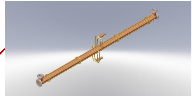
Two 3m S-band accs for linac-I 17MV/m gradient designed Outer water cooling dipole and quadrupole field exit.
