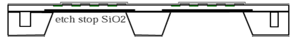
d) anisotropic deep etching opens "windows" in handle wafer
