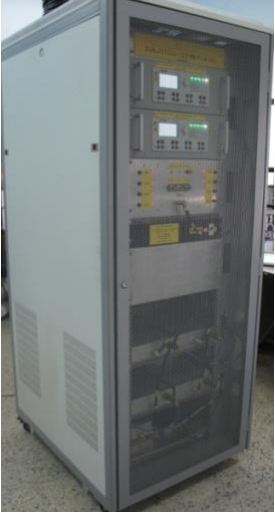
20kW SSPA Acceptance testing and Sub-harmonic buncher tests at CERN
