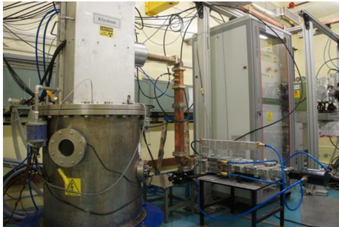
Standalone endurance tests on a microwave load.
