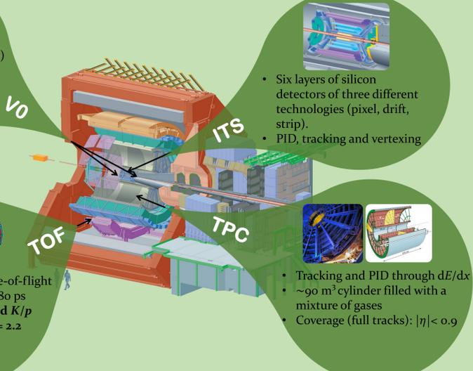
• Six layers of silicon detectors of three different technologies (pixel, drift, strip).
