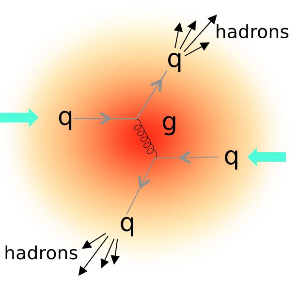
Partons originating from an initial hard collision lose energy in the created medium before forming hadrons.
