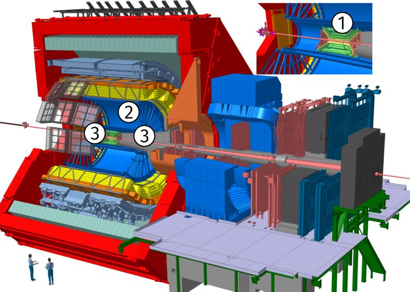
For tracking of charged particles the Inner Tracking System (**ITS**) and the Time Projection Chamber (**TPC**) are used.
