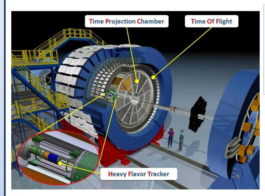
Heavy Flavor Tracker Inner tracking system (2014-2016): ♦ Silicon Strip Detector: r ~22 cm ♦ Intermediate Silicon Tracker: r ~14 cm ♦ PIXEL detector: r ~2.8 & 8 cm, MAPS,
