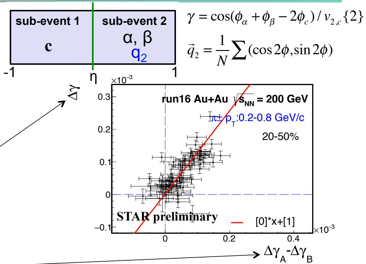
Bkg  $\Delta\gamma$  mass shape:  $\Delta\gamma_A - \Delta\gamma_B$
