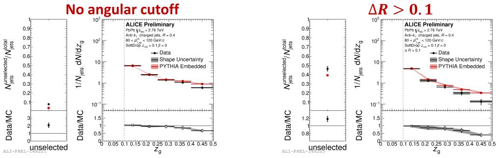
$z_g$  distribution for inclusive jet sample in Pb-Pb collisions in jet  $p_T$  range 80-120 GeV/c normalising to the total number of jets in the reconstructed  $p_T^{\text{jet}}$  bin
