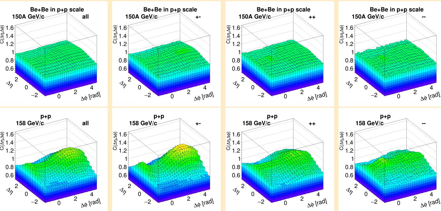
Correlation results of Be+Be are about 30% weaker than the results of p+p due to higher combinatorial background, while the mean multiplicity in the Be+Be events is about 4-5 times higher than in p+p events at the similar beam momentum.
