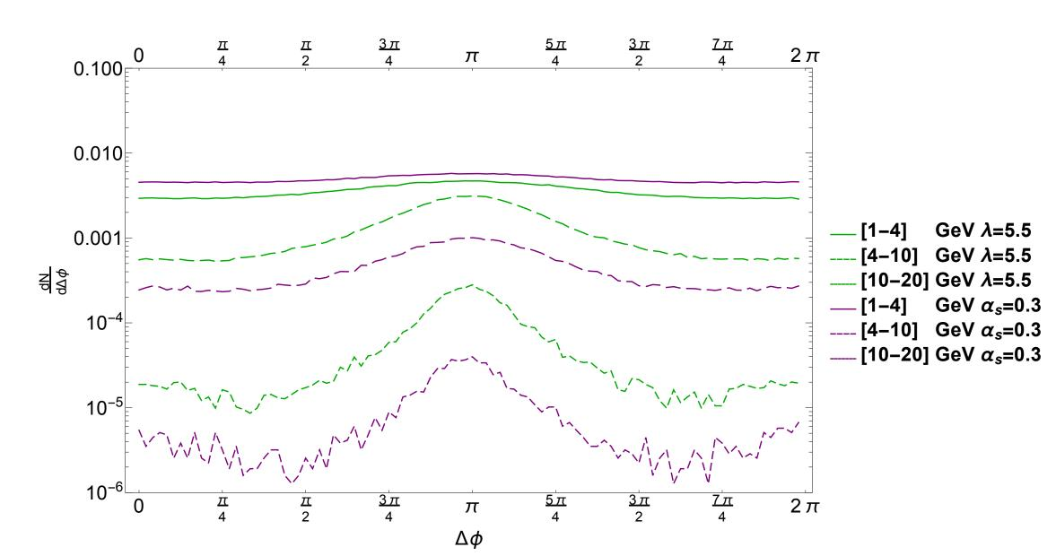
$rac{dN}{d\phi}$  correlations for NLO initialization of the D(p) model. The [1-4]GeV correlations are entirely washed out, but the signal is still observable for the higher  $p_T$  classes.
