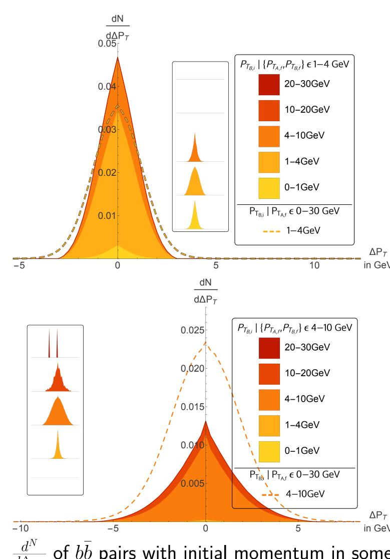
$rac{d^{r}}{d\Delta p_{T}}$  of bb pairs with initial momentum in some given class. We observe that the bulk of particles in the [1-4]GeV momentum class were initially in this class too. Hence, the order of magnitude difference to the pQCD momentum correlations must be due to weaker correlation of low momentum bottom quarks in the weakly coupled plasma.
