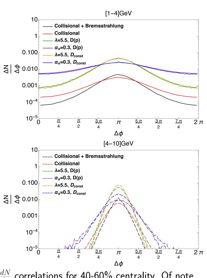
$\frac{dN}{d\phi}$  correlations for 40-60% centrality. Of note is the order of magnitude difference between the strong and weak coupling based correlations in the [1-4]GeV momentum class. Naïvely, one may expect this difference to be caused by more efficient suppression of high  $p_T$  particles in the strongly coupled plasma, but as the inital momentum correlations show, this is not the case.
