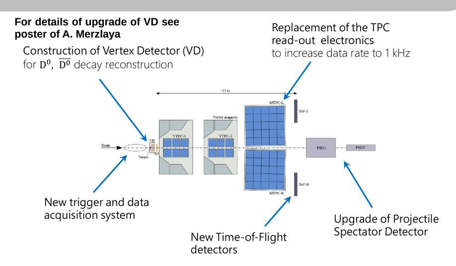
Upgrades are needed to increase rate capability of NA61/SHINE by one order of magnitude to 1 kHz
