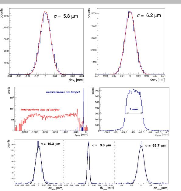
Spacial resolution of the sensor < 5µm as expected
