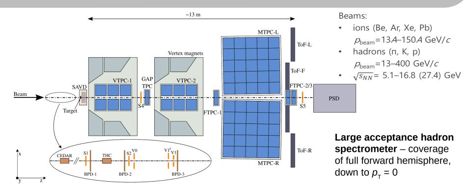
**Beam detectors and triggering** → a set of upstream scintillator and Cherenkov counters and beam Position detectors provides timing reference, charge and position measurements
