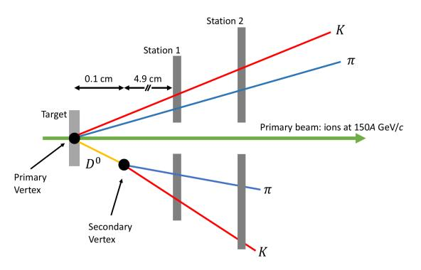
Vertex detector is needed to reconstruct **primary vertex** and **secondary vertexes** with high precision.
