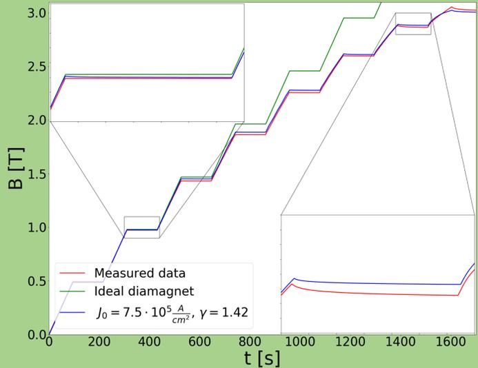
accurately using the eddy current model. The tested tube could perfectly shield about 3 T outer[4] field with 8.5 mm wall thickness.
