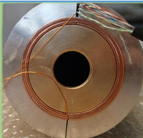
Four Hall sensors were placed on the outside and in the inside of the shield parallel with the outer magnetic field. Another two were placed inside perpendicularly.
