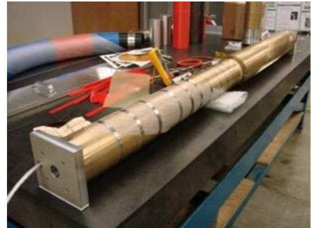
CCT winding and assembly, courtesy LBNL.
