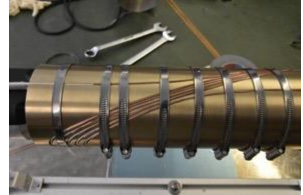
Preparation for heat treatment.
