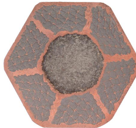
Hexagonal composite rod (subelement) consists of axial Sn alloy rod, 6 sectors composed by the Nb(Ti) doped filaments embedded into Cu matrix and separated by the Cu layers
