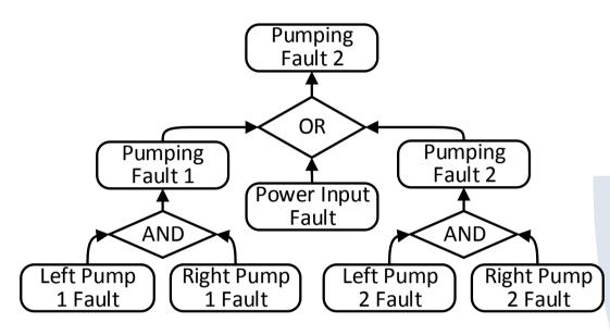
Fault tree model of each subsystem
