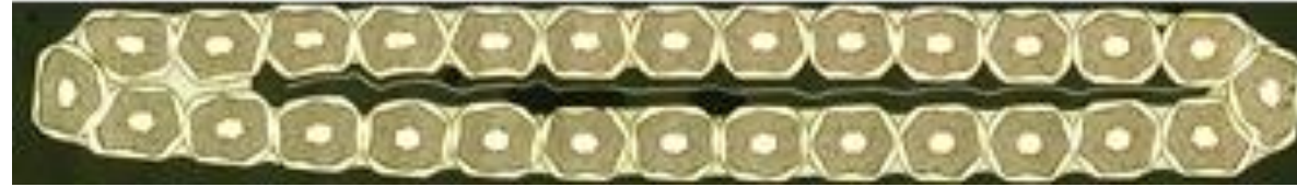
1 mm RRP150/169 28-strand cable with SS core
