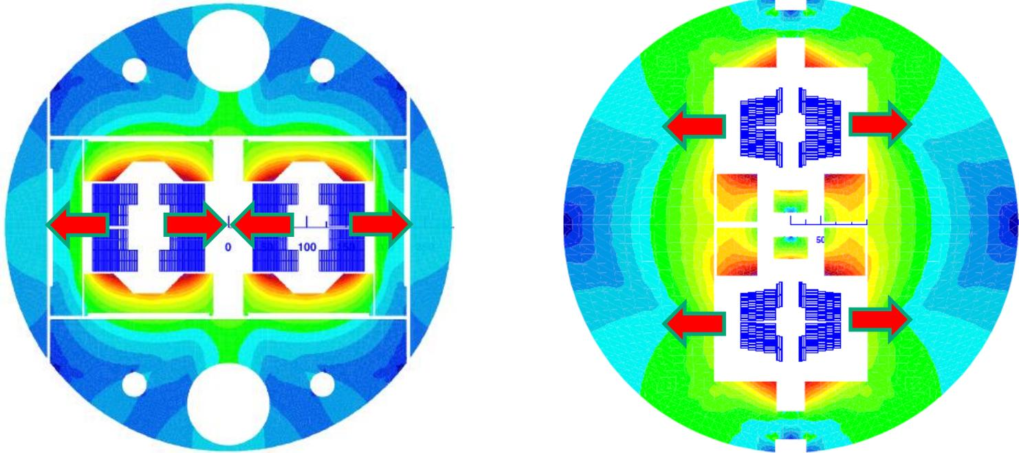
The forces per quadrant are similar for the block and common coil designs. However, the **external support structure** needs to hold **twice** the force in the case of the common coil magnet.
