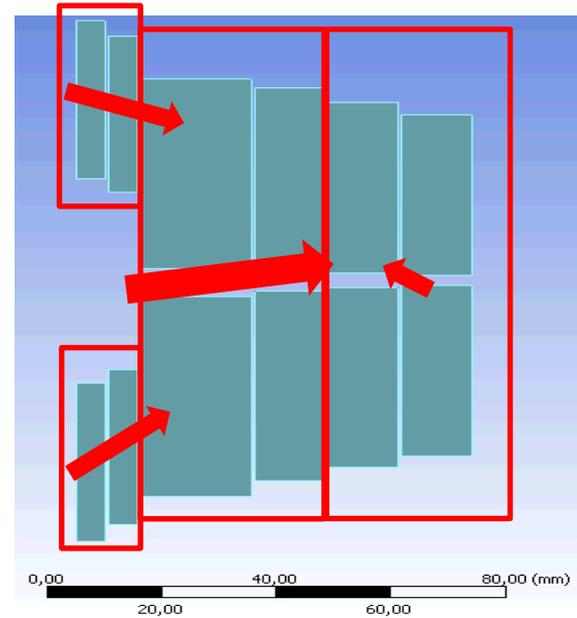
The forces per coil are similar for the block and common coil designs. In the case of the common coil, there is a **vertical repulsive force** between both apertures.
