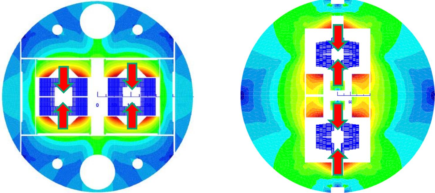
In a block dipole, the shell can apply a direct vertical pre-stress on coils.
