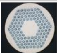
0.7 mm RRP108/127 40-strand cable with SS core
