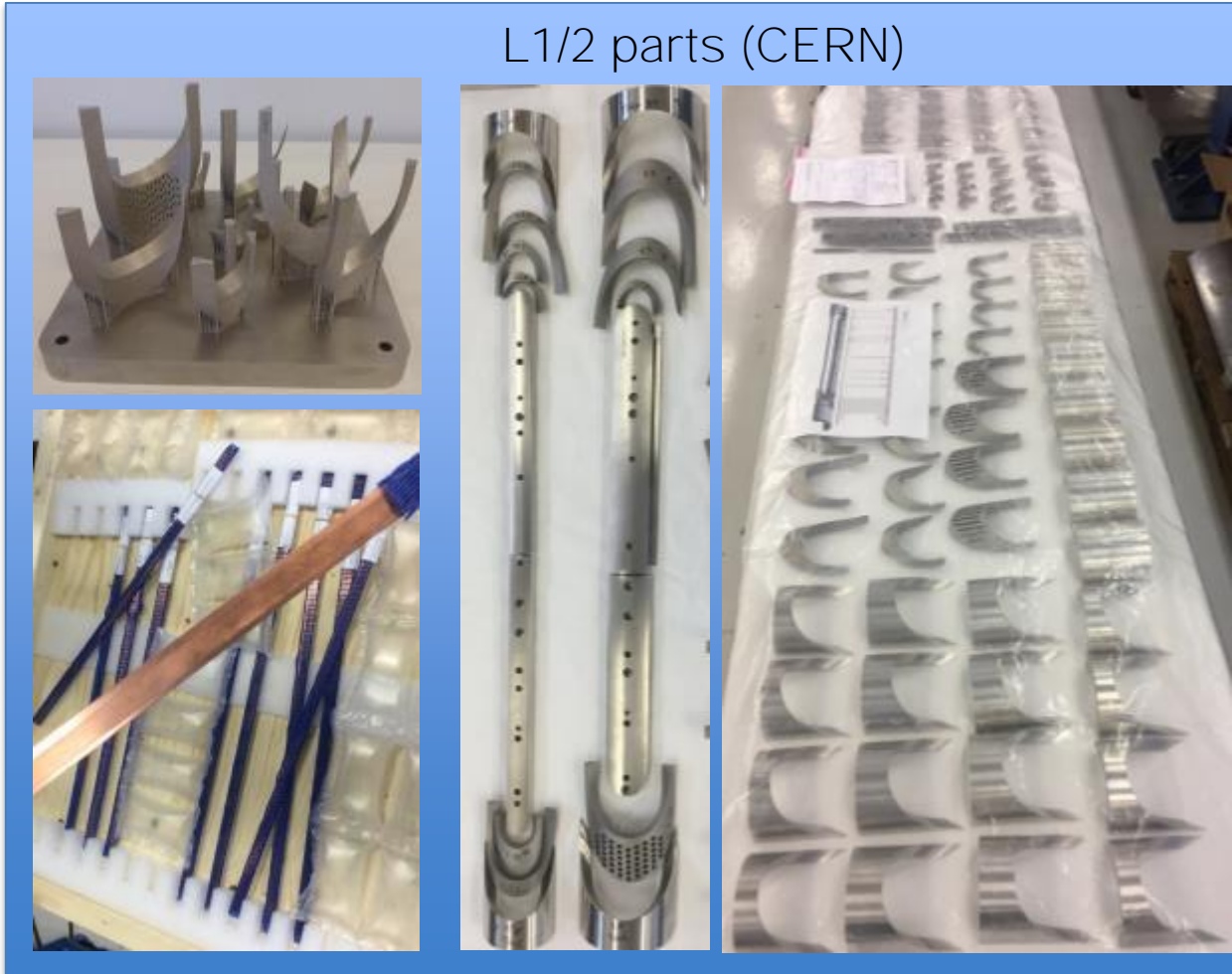
Ti and Glidcop Wedges Ti poles and spacers, SS saddles
