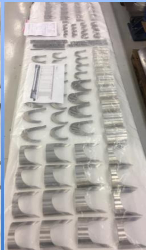
Ti poles and spacers, SS saddles
