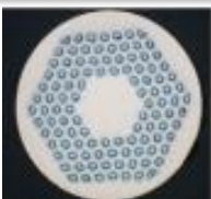
0.7 mm RRP108/127 40-strand cable with SS core
