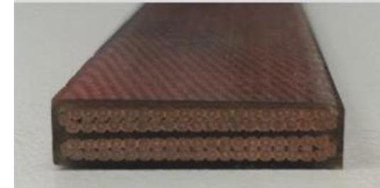
FRESCA sample, RRP – Nb<sub>3</sub>Sn 11T cable stack
