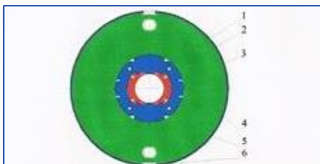
Fig.1. Design I: 1 – coil; 2 – collars; 3 – key; 4 – iron yoke; 5 – outer shell; 6 – staple.
