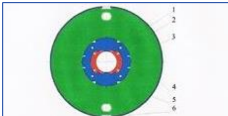
Fig.1. Design I: 1 – coil; 2 – collars; 3 – key; 4 – iron yoke; 5 – outer shell; 6 – staple.
