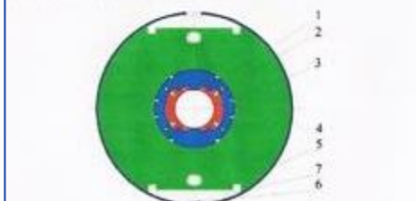
Fig.2. Design II: 1 – coil; 2 – collars; 3 – key; 4 – iron yoke; 5 – outer shell; 6 – staple; 7 – C-clamp.
