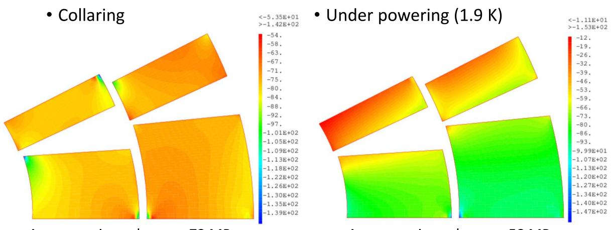
Average azimutal stress: 73 MPa
